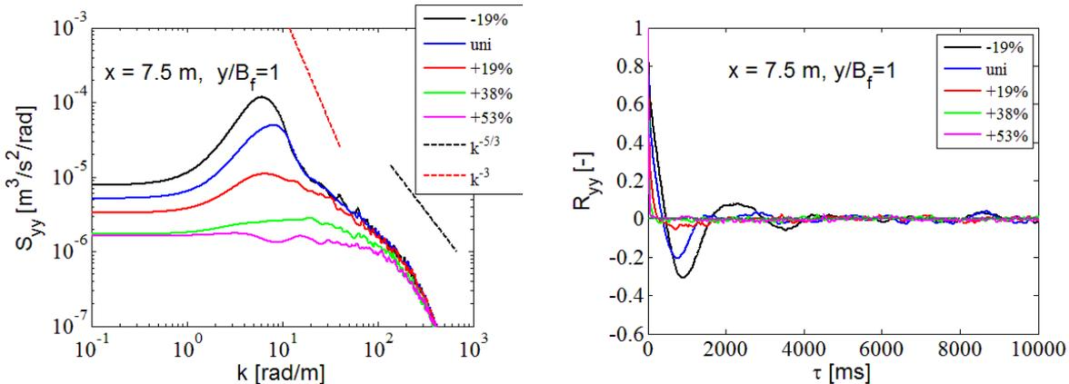
Figure 4. LNEC,  $D_r \sim 0.2$ . Power density spectra of lateral velocity fluctuation,  $S_{yy}$ , and temporal auto-correlation function  $R_{yy}$ . Measurements at the junction MC/FP ( $y/B_f = 1$ , i.e. top of the sloped bank in the MC)
