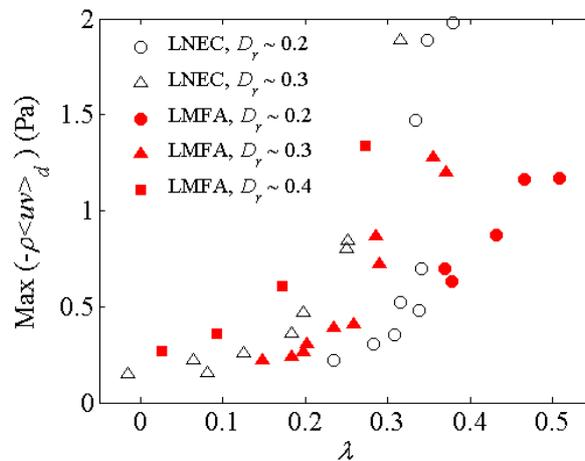
Figure 1. Peak values of depth-averaged Reynolds-stress,  $\text{Max}(-\rho\langle uv \rangle_d)$ , against velocity ratio,  $\lambda$ . LNEC flume: measurements at downstream distances  $x = 5$  and  $7.5$  m. LMFA flume, measurements at  $x = 4.5$  and  $6.5$  m.
