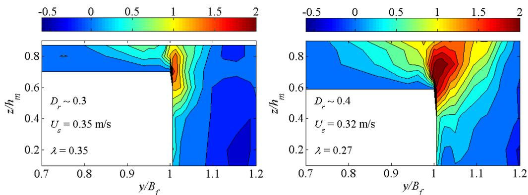
Figure 2. Effect of flow confinement: cross-sectional distribution of scaled Reynolds stress  $-\langle uv \rangle / U_s^2$ . Cases  $\Delta Q_f / Q_f^H = -19\%$ ,  $x = 4.5$  m at LMFA.  $y$ -axis is the lateral direction,  $z$ -axis is the vertical direction and  $B_f$  is the width of the FP.
