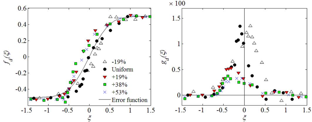
Figure 3. Scaled depth-averaged mean velocity profiles,  $f_d(\xi)$ , and scaled depth-averaged Reynolds-stress profiles,  $g_d(\xi)$ . LNEC,  $D_r \sim 0.2$ ,  $x = 7.5$  m. The error function is a usual approximation for free mixing layer velocity profile.
